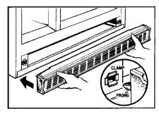
To replace base grille, align prongs on back of grille with clamps in cabinet and-push forward until the grille snaps into place.
