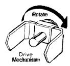
If bin does not go all the way back, remove it and rotate the drive mechanism 1/4 turn. Then push bin back again until the tab on the bin locks into the slot in the shelf.
