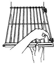
1. While pressing tabs on shelf supports on right wall, lift shelf out of grooves in supports.
