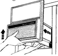
Lift the left corner to free the bin from the shelf, and pull the bin straight out while supporting it at front and back.
