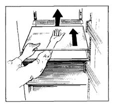
3. Pull the drawer partway out. Reach in, push the rear of the glass up; at the same time, push it back until it clears front-corner retainers.
