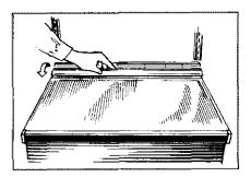
2. Put your fingers behind the gasket at the rear of the drawer and pull forward. Remove the gasket.
