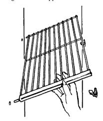
2. Pull shelf sideways until rods come out of **holes** on left wall.
