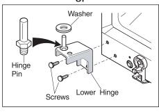
do not tighten. Hinges will have to remain loose against cabinet to align door.
