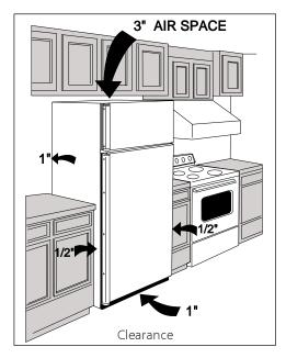
Proper air circulation and leveling will ensure efficient operation.
