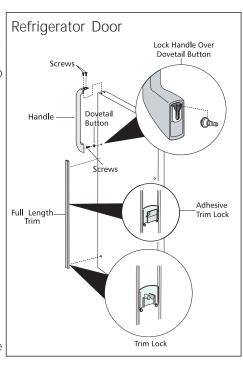
over dovetail button, swing handle into an upright position and push downward, locking it into place. Secure top of handle with screws.
