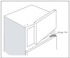
5. Carefully remove the hole plugs from the hinge holes in the center mullion and top of cabinet and reinstall in the opposite set of holes.
