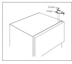
4. Remove hinge pin, hinge, and the two screws attaching the lower hinge. Save the hinge, hinge pin, washer (some models) and screws for reassembly later.
