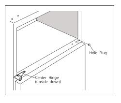
11. Place original washer (some models) over hole in refrigerator door and line up hole in center hinge. Insert hinge pin through both holes. Place washer (some models) on hinge pin, then position freezer door on center hinge.
