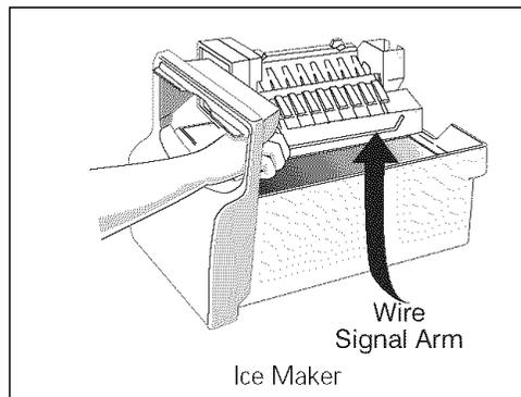
To stop the ice maker, lift the wire signal arm until it clicks, and locks in the "up" or OFF position.
