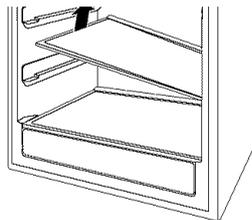
Tilt the shelf at an angle while removing or replacing
