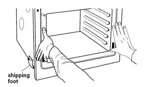
Push against seal area of front frame to push oven into cabinet until shipping feet almost contact cabinet. Use a Phillips screwdriver to remove screws attaching shipping feet. Remove and discard shipping feet.
