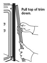
**3** Remove trim screws attaching right and left side trim to oven. Grasp the bottom end of trim and pull away from oven. Slide top end of trim downward to remove trim from oven. Take care not to scratch other surfaces with ends of trim. Set trim and screws aside on protected surface.
