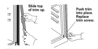
■ Slide top end of each trim upward onto oven side rails. Push each trim into place at bottom of trim. Use screws to attach each trim to oven. Take care not to scratch other surfaces with ends of trim.
