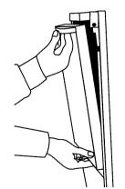
■ Completely open lower oven door. Insert small end of a door removal pin into each door hinge. Grasp door handle from the bottom and gently close door as far as it will shut. Lift slightly and grasp bottom of door with other hand. Pull door out at bottom to remove. Set door aside on protected surface.
