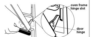
Replace the single or upper oven door by inserting ends of hinges into hinge slots in oven frame. Push behind each hinge so that hinges are pushed into oven frame as far as they will go. Open door and remove both door removal pins. Close and open door to check that door closes and opens completely. If door does not close or open completely, you have not pushed hinges completely into frame. Repeat door removal step and reinsert door into hinge slots again.
