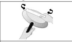
Pans should have flat bottoms. Check for flatness by rotating a ruler across the bottom. There should be no gaps between the pan and ruler.
