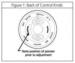
The temperature in the oven has been set at the factory. When first using the oven, be sure to follow recipe times and temperatures. If you think the oven is too hot or too cool, the temperature in the oven can be adjusted. Before adjusting, test a recipe by using a higher or lower temperature than the recommended temperature. The baking results should help you to decide how much of an adjustment is needed.
