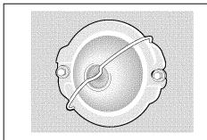
**A CAUTION** Be sure the oven is unplugged and all parts are COOL before replacing the oven light. Wear a leather-faced glove for protection against possible broken glass.
