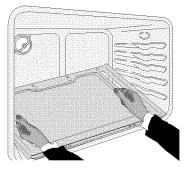
Use the finger openings along the outside edges of the oven bottom to raise and lower the oven bottom.
