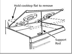
**A WARNING DO NOT** turn the burners on when the cooktop is raised for cleaning. Be sure that the top is completely lowered and securely in place before turning on the burners.
