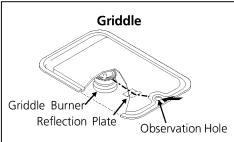
The hole in the griddle cover should be toward the backguard.
