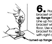
■ Place anti-tip bracket on floor with turnedup flange facing the front. Line up holes in anti-tip bracket with holes drilled in floor. Use screws to attach bracket to floor. Repeat with right anti-tip bracket.
