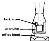
If oven flame needs to be adjusted, locate the air shutter near the center rear of the range. Loosen screw and adjust the air shutter until the proper flame appears. Tighten screw.
