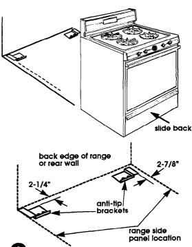
Unfold paper template and place it flat on the floor with the back and side edges positioned exactly where the back and sides of range will be located when installed.
