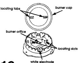
Align locating tabs on burner caps with locating slots in burner base. Burner cap should be level when properly positioned. Place burner grates over burners and caps.
