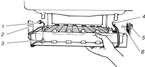
1. Cutter Grid Harness      4. Ice Level Sensor Harness
