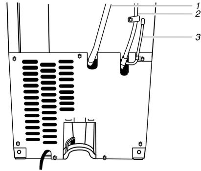
1. Drain Hose (Drain Pump models only)
