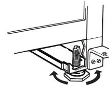
4. Use a carpenter's level to re-check the ice maker to see that it is even from front to back and side to side. If the ice maker is not level, repeat Steps 2 and 3. If the ice maker is level, go to the "Water Supply Connection" section.
