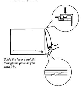
D Secure the front grille to the case by replacing the screw removed in Step 3A. If a screw was not removed in Step 3A, secure the grille to the case with a Type D screw.
