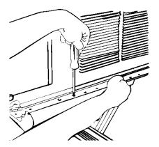
Adjust the type C leveling bolts against the outside wall so that the case has a slight tilt to the outside. Use a level; about a 1/2 bubble will be the correct case slant to the outside.
