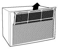
Grab the tabs on the filter and pull it up and out.
