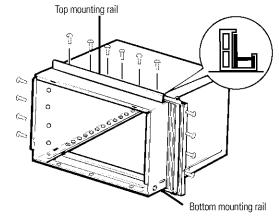
Insert the frames for the accordion panels into the top and bottom mounting rails. Attach the accordion panels to the side of the case using 8 type A screws.
