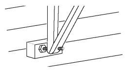
**NOTE:** Use a wood block between the leveling bolts and the wall if the wall is weak or if the weight of the air conditioner falls between the studs in the wall.
