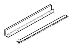
**B** Install the top mounting rail with 6 type A screws from the outside of the case.
