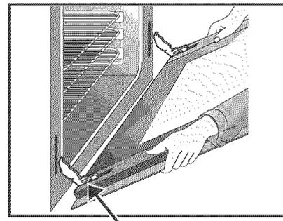
HINGE SLOT - Door removed from the appliance
