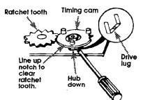
3. Insert a narrow, flat-blade screwdriver under the timing cam near the clock shaft. Gently lift cam straight up and off shaft making sure that the "V"-shaped notch clears the ratchet tooth.
