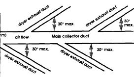
Back draft damper kits (Part No. 3391910) are available from your Whirlpool dealer and should be installed in each dryer exhaust duct to prevent exhausted air from returning into the dryers and to keep the exhaust in balance within the main exhaust duct. Unobstructed air openings are required.
