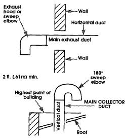
**Do Not** install screening or cap over end of duct.
