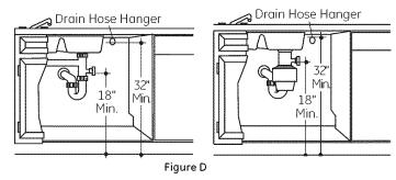
Method 2 – "High Drain Loop" with Waste Tee or Disposer
