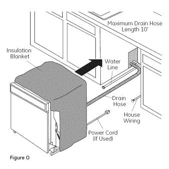
**Tip:** Position water line and house wiring on the floor to avoid interference with base of dishwasher.
