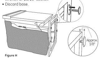
• Screw leveling legs back into the dishwasher frame, approximately 1/8" from frame as shown.
