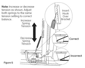
**Tip:** If door spring adjustment is necessary, check door opening and closing. If door does not open easily or falls too quickly, check spring cable routing. The cable is held in place by "shoulders" on the pulley. Check to be sure cable has not slipped over the pulley shoulders.
