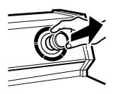
**NOTE:** To **stop** the washer at any time, push in the Cycle Control knob. To **restart** the washer, close the lid (if open) and pull out the Cycle Control knob.
