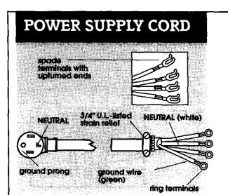
Four-wire power supply cord must have four, No.-10 copper wires and match a four-wire receptacle of NEMA Type 14-30R. The fourth wire (ground conductor) must be identified with a green cover and the neutral conductor by a white cover.
