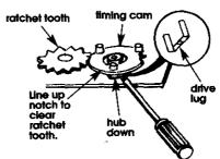
Insert a narrow, flat-blade screwdriver under the timing cam near the clock shaft. Gently lift cam straight up and off shaft making sure that the "V" -shaped notch clears the ratchet tooth.
