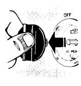
1. Pull out the center of the Oven Temperature Control.
