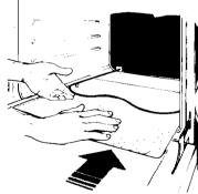
Slide the foil under the bake element.
