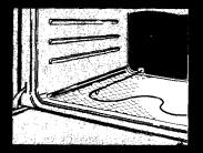
Use foil on the oven bottom only as suggested on page 12. Shock or fire hazard can result from improper use.
