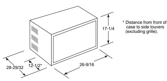
**Note:** When installing units in through-the-wall applications, keep louvers free. Do not restrict air flow areas. Fixed chassis units are not designed for through-the-wall applications.
