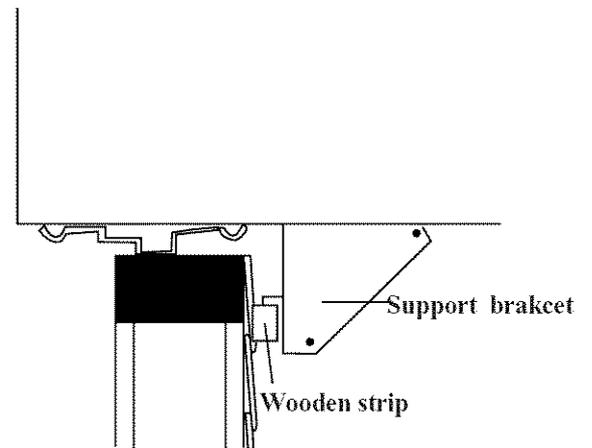
5. Screw or nail cabinet wooden frame using shims if frame is oversized, to eliminate distortion. Remember to maintain proper slope as described in Step 3.
