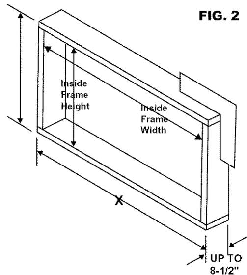
4. Build a wooden frame with the INSIDE dimensions of your model listed above. (Measure twice remember...) Frame depth should be the same as wall thickness. Fill in the space from the opening to the studs with wood spacers, as shown.
