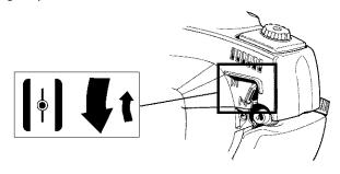
**Air purge:** Press the air purge diaphragm repeatedly until fuel begins to fill the diaphragm. The diaphragm need not be completely filled.
