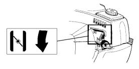
**Air purge:** Press the air purge diaphragm repeatedly until fuel begins to fill the diaphragm. The diaphragm need not be completely filled.
