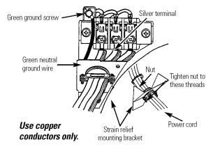
Attach the power cord neutral (center wire) conductor to the silver-colored center terminal on the terminal block. Tighten the screw securely.
