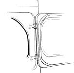
Remove 4 screws-one from each hinge first
