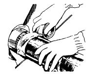
Attach exhaust duct to each dryer duct. Then connect exhaust ducts to exhaust hoods or main exhaust. Use duct tape to seal all joints.
