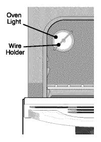
On some models, the oven light automatically turns on when the door is opened. Some models have a switch located on the control panel to turn on the light. The oven light is located at the rear of the oven and is covered with a glass shield held by a wire holder. The glass shield must be in place whenever the oven is in use. **To replace the oven light:**
