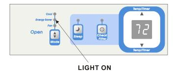
**NOTE**: In this mode, the fan will continue to run for 3 minutes after the compressor shuts off. The fan then cycles on for 2 minutes at 10 minute intervals until the room temperature is above the set temperature, at which time the compressor turns back on and cooling starts.
