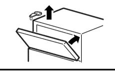
**6.2.3.** Make sure the door is slightly above the top of the cabinet and the gap between the doors is even across the front. Tighten the top hinge screws. Do not overtighten these screws–tighten them until they are just snug, then turn them another one-half turn.
