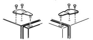
Installing the hinge on the left. Installing the hinge on the right.
