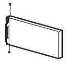
**5.4.3** Remove the screw from the right top edge of the door and insert it into the handle screw hole on the left side.
