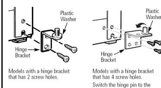
4.3 Interchange hinge (and the shim glued to it) and screws at top right with screws at top left of cabinet.Do not tighten screws on hinge side at this time.
