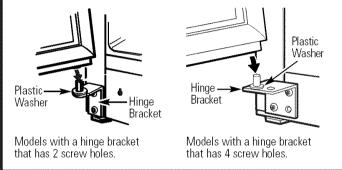
6.1.2 Insert the pin on the center hinge into the socket in the top of the door. Place the spacer, then the washer, on the hinge pin.NOTE: The center hinge must be turned over as shown when mounted on the left side.
