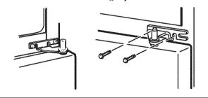
**3.3** Remove the tape and tilt the door away from the cabinet. Lift the door from the pin in the bottom hinge bracket. (If the plastic washer sticks to the door bottom, put it back on the hinge.)
