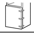
**3.2** Using a 5/16" hex-head socket screwdriver and a 5/16" open-end wrench, remove the two screws holding the center hinge (and the shim glued to it) to the cabinet. Lift the center hinge to free its pin from the socket in the top of the door, and set hinge and screws aside. **Be careful not to lose the center hinge spacer and washer.**
