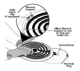
**ACAUTION** Be sure the range is cool before removing elements or drip bowls. Be careful not to bend terminal ends when replacing elements after cleaning.
