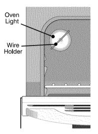
For models equipped with the interior oven light, the light bulb is located at the rear of the oven and is covered with a glass shield held by a wire holder. The glass shield must be in place whenever the oven is in use.
