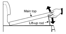
**ACAUTION** When lowering the lift-up range top, grasp the sides with finger-tips only. Be careful not to pinch fingers. **DO NOT** drop or bend the range top when raising or lowering. This could damage the surface.
