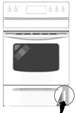
Serial plate location; Open storage drawer (some models) or remove outer lower panel (some models).
