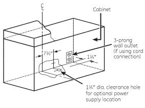
**NOTE:** If using optional Power Cord Kit JXHC1, feed the power cord through the hole in the top cabinet while raising the hood. Loop any excess length of cord and tie away with a suitable tape or tie.
