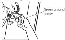
AWARNING: IMPROPER CONNECTION OF ALUMINUM HOUSE WIRING TO THESE COPPER LEADS CAN RESULT IN A SERIOUS PROBLEM. <u>USE ONLY CONNECTORS DESIGNED FOR JOINING COPPER TO ALUMINUM</u> AND FOLLOW THE MANUFACTURER'S RECOMMENDED PROCEDURE CLOSELY.
