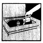
4. Run the washer through a complete cycle with one cup of detergent to clean out the antifreeze.
