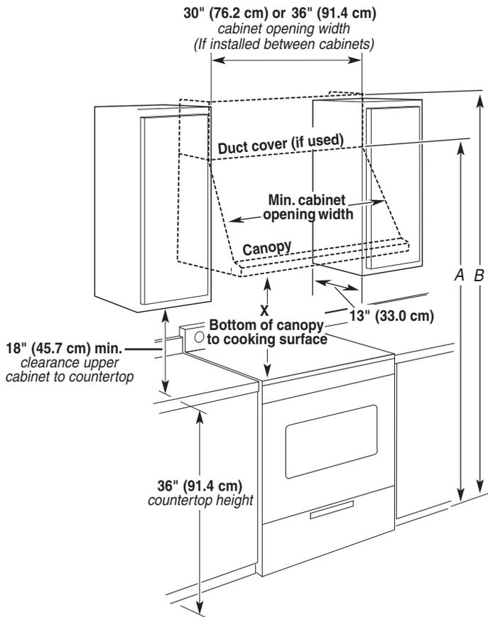
A. For installations with canopy only. 70" (177.8 cm) minimum above electric cooking surface. 76" (193.0 cm) minimum above gas cooking surface.
