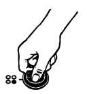
2. Lift the edge of the unit, opposite the receptacle, just enough to clear the element hold-down clip and the reflector bowl.
