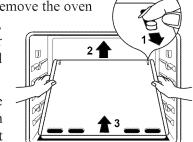
edge of the oven bottom clears the oven front frame. Remove oven bottom from oven.
