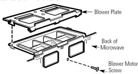
**5** Carefully pull out the blower unit. The wires will extend far enough to allow you to adjust the blower unit.
