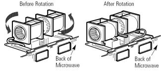
**4** Gently remove the wires from the grooves. Reroute the wires through grooves on other side of the blower unit.
