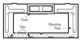
[11] Attach the other 28" foam tape to the front of the mounting plate around both of the exhaust openings where it will touch the microwave.
