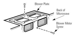
**8** Replace the blower plate in the same position as before with the screw.
