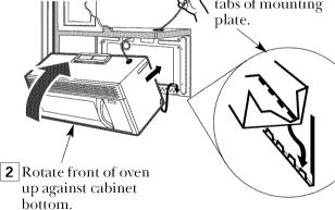
Insert a self-aligning screw through top center cabinet hole. Temporarily secure the oven by turning the screw at least **two full turns** after the threads have engaged. (It will be completely tightened later.) Be sure to keep power cord tight. Be careful not to pinch the cord, especially when mounting flush to bottom of cabinet.
