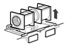
**6** Roll the blower unit 90° so that fan blade openings are facing toward the front of the microwave.
