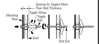
Place the mounting plate against the wall and insert the toggle wings into the holes in the wall to mount the plate.
