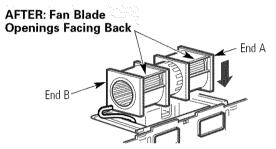
CAUTION: Do not pull or stretch the blower unit wiring. Make sure the wires are not pinched.
