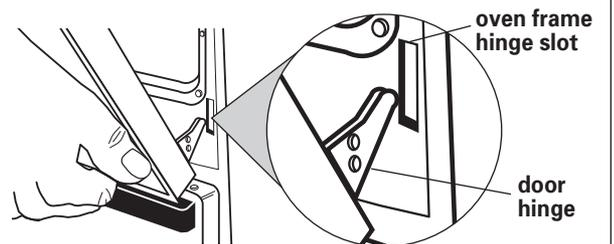
**9.** Replace the single or upper oven door by inserting the ends of hinges into hinge slots in oven frame. Push behind each hinge so that hinges are pushed into oven frame as far as they will go. Open door and remove both door removal pins. Close and open door to check that door closes and opens completely. If door does not close or open completely, you have not pushed hinges completely into frame. Repeat door removal step and reinsert door into hinge slots again. Repeat for lower oven door.
