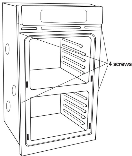
**6.** Important: Securely fasten oven to cabinet using the screws provided (two screws for a single oven or four screws for a double oven). Insert the screws through holes in mounting rails. Do Not overtighten screws.
