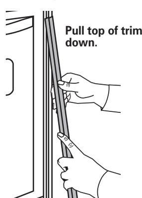
**3.** Remove trim screws attaching right and left side trim to oven. Grasp the bottom end of trim and pull away from oven. Slide top end of trim downward to remove trim from oven. Take care not to scratch other surfaces with ends of trim. Set trim and screws aside on protected surface.
