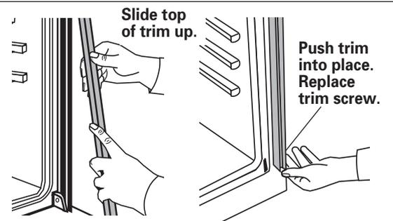
**7.** Slide top end of each trim upward onto oven side rails. Push each trim into place at bottom of trim. Use screws to attach each trim to oven. Take care not to scratch other surfaces with ends of trim.
