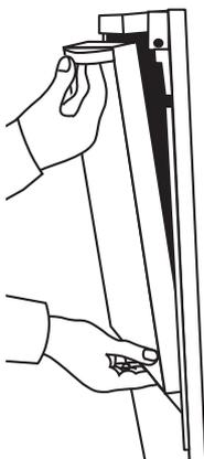
**2.** Completely open lower oven door. Insert small end of a door removal pin into each door hinge. Grasp door handle from the bottom and gently close door as far as it will shut. Lift slightly and grasp bottom of door with other hand. Pull door out at bottom to remove. Set door aside on protected surface. Repeat for upper oven door.
