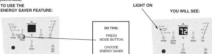
Note: In this mode, the fan will continue to run for another 3 minutes after the compressor shuts off. The fan then cycles on for 2 minutes at 10 minute intervals until the room temperature is above the set temperature, at which time the the cooling system turns back on.
