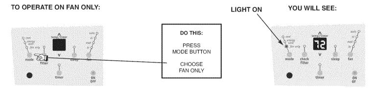
**Note:** Use this function only when cooling is not desired, such as for room air circulation or to exhaust stale air. (Remember to open the vent during this function, but keep it closed during cooling for maximum cooling efficiency.) You can choose any fan speed you prefer. (Except "Auto Fan").
