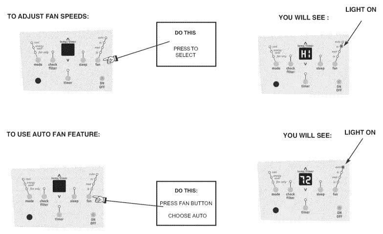
**Note:** Fan speed starts at High Speed and adjusts to a slower speed as the room temperature dictates. For example if the room doesn't get too warm, it will stay at the slowest speed. If the room temperature rises quickly, such as a door being opened, it will automatically go to the highest speed. The fan speeds will re-adjust back to the slowest speed as the room returns to the original set temperature.
