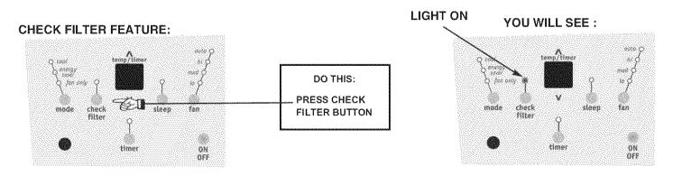
Note: This feature is a reminder to clean the Air Filter (See Care and Cleaning) for more efficient operation and cooling. The LED (light) will illuminate after 250 hours of operation. To reset after cleaning the filter, press the "Check Filter" button and the light will go off.
