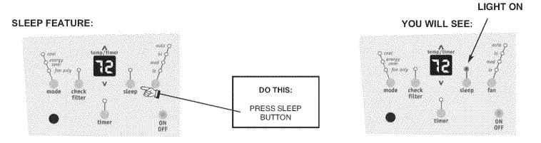
**Note:** In this mode the set temperature will increase by 2° F 30 minutes after the mode is selected. The temperature will then increase by another 2° F after an additional 30 minutes. This new temperature will be maintained for 7 hours before it returns to the originally selected temperature. This ends the "Sleep" mode and the unit will continue to operate as originally programmed. The "Sleep" mode program can be cancelled at any time during operation by pressing the "Sleep" button again.
