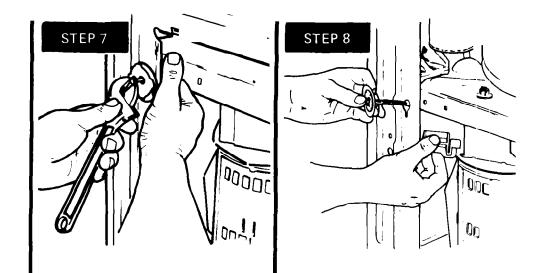
By hand, turn each of the front leveling legs half way (up to the diamond marking on the threads) into the front cabinet gussets. Liquid detergent can be used to reduce the force needed to turn the legs into the gussets.
