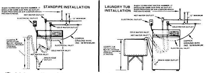
\*The drain hose assembly must fit in the standpipe so that there is an air gap around the drain hose inside the standpipe. A snug fit can cause a siphoning action.
