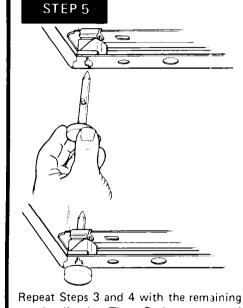
Repeat Steps 3 and 4 with the remaining rear leveling leg. Then: Push up on one of the rear leveling legs and then on the other to check to see if the self-leveling legs are working properly. If they are not working properly, recheck steps 3, 4 and 5 to make sure you have properly followed the instructions in those steps. STEP 6
