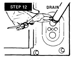
Place the drain hose in the laundry tub or standpipe, measure and cut for proper length. Secure to the angle connector with the larger hose clamp. DO NOT KINK HOSES. Now replace service panel. A complete typical installation is shown on page 11 of this instruction.
