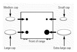
Make sure that the heads and caps are replaced in the correct locations.
