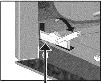
Lock engaged for door removal
