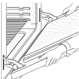
HINGE SLOT - Door removed
