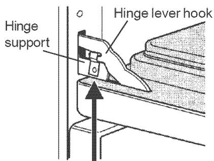
Lock engaged for door removal
