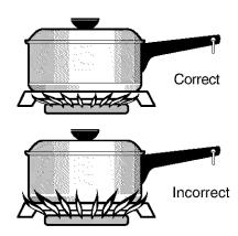
Never extend the flame beyond the outer edge of the utensil. A higher flame simply wastes heat and energy, and increases the risk of being burned by the gas flame.
