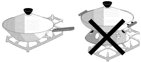
Proper use of flat-bottom wok on Surface Burner Grate Figure 2
