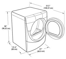
\* Most installations require a minimum 5½ in. (14 cm) clearance behind the dryer for the exhaust vent with elbow. See "Venting Requirements."
