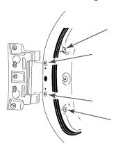
Remove the 2 screws that hold the handle bracket to the door.
