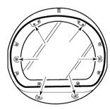
5. Lift the inner door assembly off of the outer door assembly. Set the outer door assembly aside.
