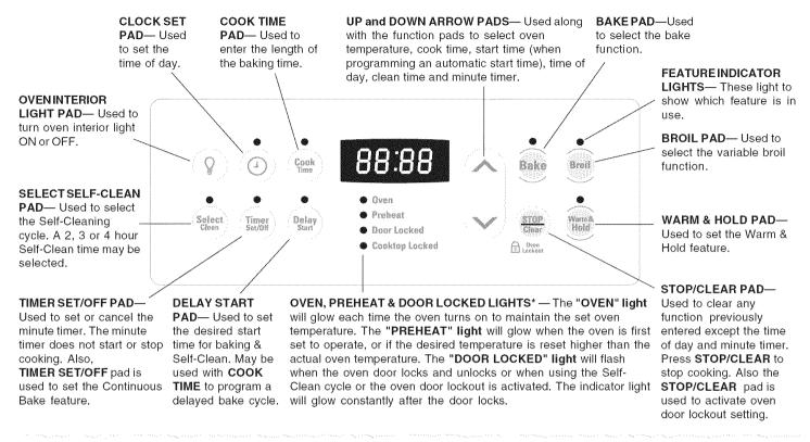
\*Note: The **OVEN** indicator light on the electronic display will turn ON and OFF when using the Bake feature and during preheat. This is normal and indicates that the oven is cycling to maintain the selected baking temperature. When the preheat indicator light turns OFF, your oven is ready.
