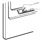
Stainless Steel: To clean stainless steel surfaces, use a damp cloth with a mild, non-abrasive cleaner suitable for stainless steel surfaces. Remove the cleaner residue, and then dry with a clean cloth.
