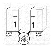
3 After leveling, verify door stop contacts lower hinge and top of door does not contact upper hinge through full movement of door (from fully closed to fully open).
