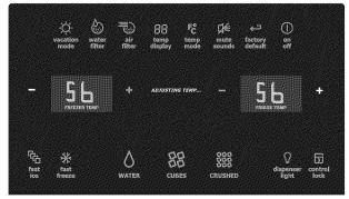
Sabbath Mode is turned ON and OFF by pressing and holding both the outermost "-" and "+" indicators for five seconds for both the Wave-Touch™ and IQ-Touch™ modes. The display shows "Sb" while in Sabbath mode.
