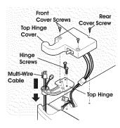
Detach the multi-wire cable connector located above the top hinge. Grasp both sides of the connector firmly and pull apart.
