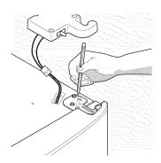
2 Remove the two screws from the top hinge. Lift the door off of the bottom hinge and set it aside.
