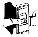
Cold air flows against the meat pan through an opening between the freezer and the refrigerator. This helps keep the meat pan colder than the rest of the refrigerator.
