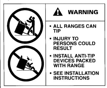
**WARNING:** To reduce the risk of tipping of appliance from abnormal usage or by excessive loading of the oven door, the appliance must be secured by a properly installed anti-tip device. When removing the appliance for cleaning, be sure the anti-tip device is engaged when the range is replaced. Look underneath range to verify that one of the rear leveling legs is properly engaged in the bracket slot. The anti-tip device secures the rear leveling leg to the floor when properly engaged.
