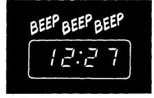
When the time is up, you will hear a beeping sound. Push the Min/Sec Timer Button to stop the beeping. The beeping will automatically stop after 1-2 minutes.
