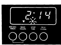
8. The Bake Hours Signal Light will stay on and the Stop Time Signal Light will flash. If you want to see the Stop Time, push the Stop Time Button. Push the Bake Hours Button to see baking time again.
