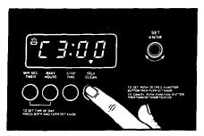
3. Push in and release the Self-Clean Button. A 3-hour Self-Cleaning cycle will be set automatically. The Display will count down the time in minutes. The Auto Oven Symbol, Self-Clean and "heating" Signal Lights will come on.
