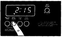
5. Set the clock for the length of baking time you want. Push in the Bake Hours Button. Turn the Set Knob until the length of baking time you want shows in the Display. This example shows 2 hours, 15 minutes. Bake Hours can be set for up to 11 hours, 59 minutes.
