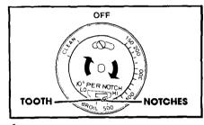
4. To raise the temperature, move a notch closer to HI. Each notch equals about 10°F (5°C).
