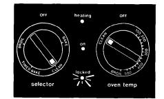
4. The "locked" Signal Light will come on when the oven temperature exceeds normal baking temperatures. The Lock Lever must not be moved and the door can't be opened when the light is on. If you want to see Stop Time of the Self-Cleaning cycle, push the Stop Time Button. Push the Self-Clean Button to see cleaning time again.
