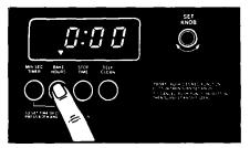
**11. To stop the oven before the preset time:** Push in the Bake Hours Button and turn the Set Knob counterclockwise until the Display shows "0:00." Turn the Oven Selector and Oven Temperature Control to OFF
