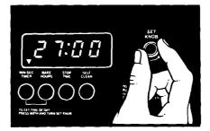
2. Turn the Set Knob until the desired time shows in the Display. Turning the knob clockwise increases the numbers, while turning the knob counterclockwise decreases the numbers.
