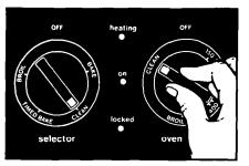
Set the Oven Selector and Oven Temperature Control on CLEAN. The "on" Signal Light will come on.
