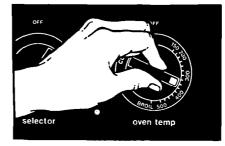
3. Set the Oven Temperature Control to the baking temperature you want. The "heating" Signal Light will come on. The oven is preheated when the "heating" Signal Light first goes off.
