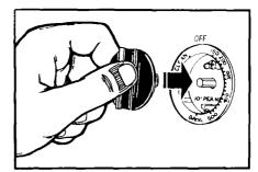
4. Push control knobs straight back on. Make sure they point to OFF.
