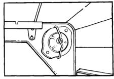
**4.** Replace the bulb cover and snap the wire holder in place. Turn the power back on at the main power supply.
