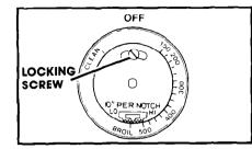
2. Loosen the locking screw. Note the position of the notches.
