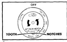
**3.** To lower the temperature, move a notch closer to LO. Each notch equals about 10°F (5°C).
