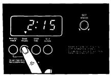
7. Set the clock for the length of baking time you want: Push in the Bake Hours Button, then turn the Set Knob until the length of baking time you want shows in the Display. This example shows 2 hours, 15 minutes. Bake Hours can be set for up to 11 hours. 59 minutes
