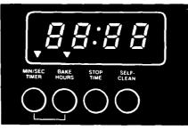
Then, 4 eights and the Min/Sec Timer and Bake Hours signal lights will flash. The flashing means that the clock is ready to be set.
