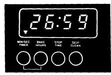
**3.** After setting the time you want, the Signal Light will stay on and the Display will start counting down in seconds.
