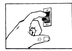
1. WARNING: To avoid possible shock hazard, turn off the electric power at the main power supply.
