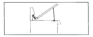
**To lower the top:** Hold the front edge of the cooktop and carefully push back on each support rod, if equipped, to release the notched support. Then gently lower the top into place. The support rods will slide into the cooktop frame.
