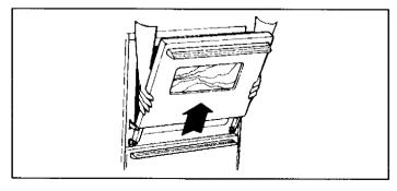
**To replace door:** Grasp the door at each side, align the slots in the door with the hinge arms and slide the door down onto the hinge arms until it is completely seated on the hinges.
