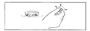
An intermediate fiame size is used to continue a cooking operation. Food will not cook any faster when a higher flame setting is used than needed to maintain a gentle boil. Remember, water boils at the same temperature whether boiling gently or vigorously.
