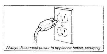
The three-prong grounding plug offers protection against shock hazards. DO NOT CUT OR REMOVE THE THIRD GROUNDING PRONG FROM THE POWER CORD PLUG.
