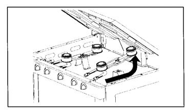
**To remove:** Allow the burner assembly to cool. Lift up cooktop. Grasp the burner assembly and rotate it slightly toward the left to release the two tabs on the assembly. Then lift the assembly and pull toward the back of the cooktop until the air shutter ends on the assembly release from the valves.
