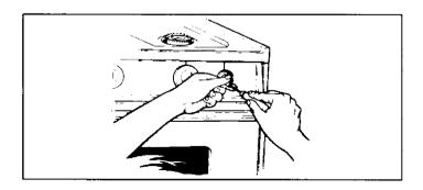
The flame must be of sufficient size to be stable on all burner ports. If the flame adjustment is needed, adjust ONLY on the LO setting. Never adjust flame size on a higher setting.
