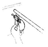
With the Thermostat knob in the OFF position, hold a lighted match to the pilot located at the back of the oven burner. Once the pilot lights, replace the broiler rack and pan or the lower panel. (NOTE: The oven burner is shown with the metal flame spreader removed from the oven burner.)
