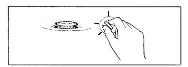
If a knob is turned very quickly from the HI to the LO setting, the flame may go out, particularly if the burner is cold. If this occurs, turn the knob to the OFF position. Wait several seconds, then light the burner again.
