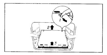
To remove: When cool, remove the oven racks. Slide the two catches, located at each rear corner of the oven bottom, toward the front of the oven. Lift the rear edge of the oven bottom slightly. Then slide it back until the front edge of the oven bottom clears the oven front frame. Remove the oven bottom from the oven.
