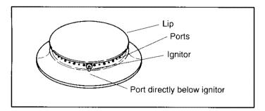
The surface burner will not light if the ignitor is damaged, broken, soiled or wet. The burner will also not light if the ports, especially the small port located directly below the ignitor, are blocked. See page 16 for cleaning instructions.
