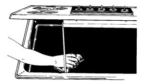
After cleaning burner box, lift cooktop slightly and disengage support rod. Pull cooktop forward slightly, without lowering it, until hinges lock. Lower cooktop until it rests on countertop. Wipe back edge of cooktop with a warm, soapy cloth, rinse and dry thoroughly.
