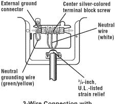
3-Wire Connection with Frame-Grounding Conductor
