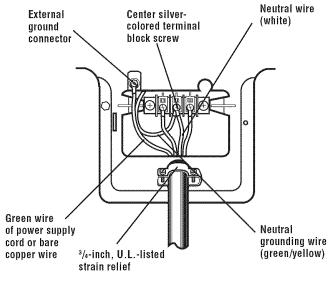
4-Wire Connection with Frame-Grounding Conductor
