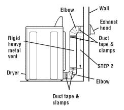
The vent usually comes in 2-foot lengths. Use tin snips to cut the vent 3 inches longer than your measurement in order to make a connection.
