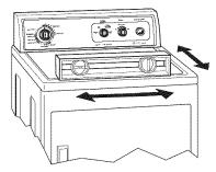
**STEP 7.** If dryer is not level, prop the dryer up using two stacked cardboard corner posts. Use a wrench to adjust the legs up or down.
