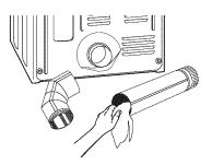
• Make sure exhaust hood is not plugged with lint. Follow the instructions in this section to reinstall your vent system.
