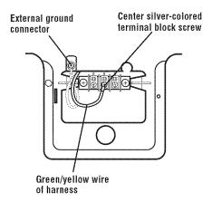
**STEP 5.** Connect neutral grounding wire and the neutral wire (white or center) of direct wire cable under the center screw of terminal block. **STEP 6.** Place the hook-shaped end of the wire over the terminal block screw. The open side of the hook should face to the right. Squeeze hook end of wire together to form a loop.
