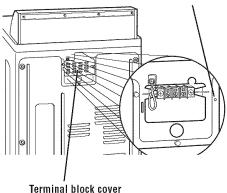
**STEP 3.** Attach a <sup>3</sup>/<sub>4</sub>-inch, U.L.-listed strain relief to the hole below terminal block opening. Strain relief should have a tight fit with dryer cabinet and be in a horizontal position. Put the direct wire cable through the strain relief.
