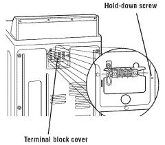
**STEP 3.** Attach a <sup>3</sup>/<sub>4</sub>-inch, U.L.-listed strain relief to the hole below terminal block opening. Strain relief should have a tight fit with dryer cabinet and be in a horizontal position. Put the power supply cord through the strain relief.
