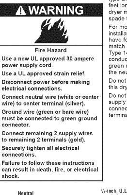
Local codes may permit the use of a U.L.-listed, 120/240-volt minimum, 30-ampere, dryer power supply cord kit (pigtail). Power supply cord should be type SRD or SRDT and be at least four feet long. The wires that connect to the dryer must end with ring terminals or spade terminals with upturned ends.
