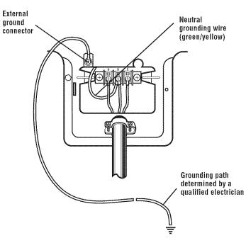
Alternate 3-Wire Connection with External-Grounding Conductor
