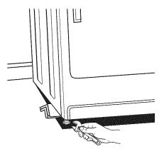
**NOTE:** It may be necessary to level the dryer again after it is moved into its final position.
