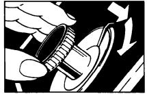
A. Push in the Control Knob and turn it to the right. It must be pushed in and turned only to the right (clockwise).
