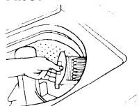
Water runs through the lint filter whenever the washer agitates. Check it often to make sure it's clean and filtering at its best.
