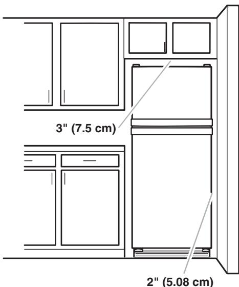
To ensure proper ventilation for your refrigerator, allow for a 1/2 in. (12.70 mm) space on each side. Allow 3 in. (7.5 cm) of space between overhead cabinets and refrigerator top. Allow at least 1 in. (25.40 mm) between back of cabinet and the wall. If your refrigerator has an ice maker, make sure you leave some extra space at the back for the water line connections.
